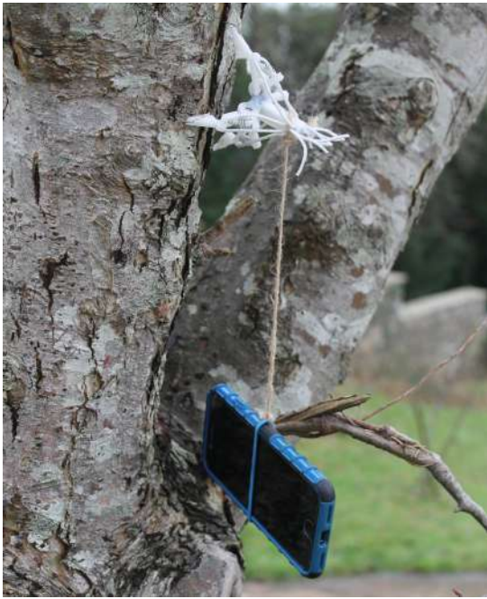
Fig. 4: Spring-loaded claw payload testing with 250g at \angle > 90^\circ
