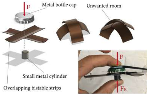
Fig. 8: Initial bistable claw design - crossover mechanism deployed by pushing into the steel concave.
