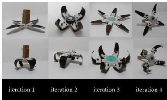
Fig. 10: Rapid iterations of the latching claw - to explore the effects of varying parameters.
